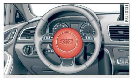
Fig. 117 Location of driver airbag: in steering wheel
