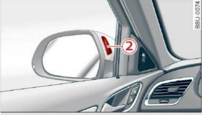
Fig. 80 Display on the exterior mirror
