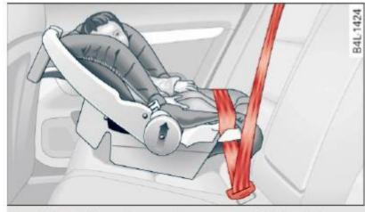
Fig. 126 Schematic overview: rearward-facing infant seat, properly installed on the rear seat
