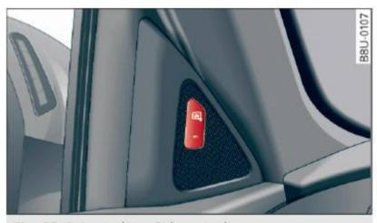
Fig. 83 Driver's door: Side assist button
