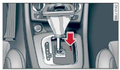
**Fig. 91** Selector lever: using the emergency release to move out of the Park position
