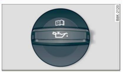
Fig. 147 Engine compartment: Cover on the oil filler neck
