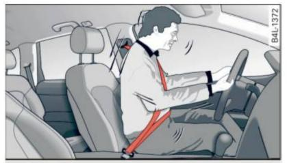
Fig. 111 Driver is correctly restrained in a sudden braking maneuver
