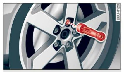
Fig. 167 Changing a wheel: using the hexagonal socket (with the blade removed) to turn the bolts
