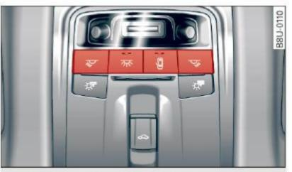
Fig. 38 Front headliner: interior lighting controls
