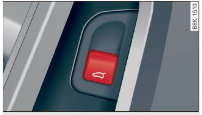
Fig. 26 Driver's door: remote rear lid release
