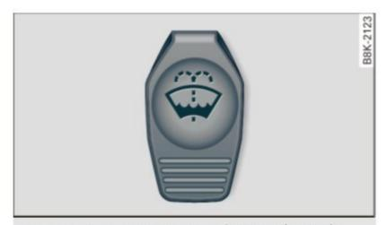
**Fig. 151** Engine compartment: Cover on the windshield washer fluid container
