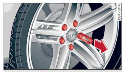
Fig. 163 Changing a wheel: removing the wheel bolt caps
