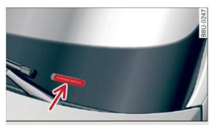
Fig. 180 Location on driver's side dash panel: Vehicle Identification Number (VIN) plate
