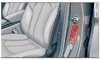
Fig. 152 Tire pressure label: located on driver's side Bpillar
