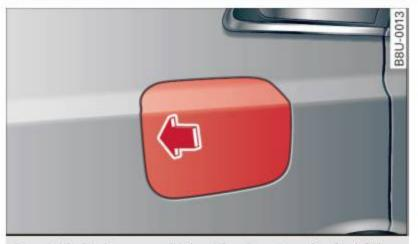
Fig. 140 Right rear vehicle side: Opening the fuel filler flap
