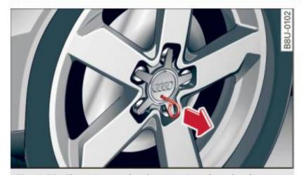
Fig. 162 Changing a wheel: removing the wheel cover
