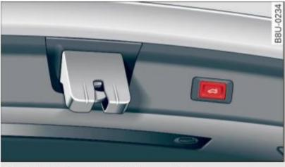
Fig. 27 Closing button in the rear lid
