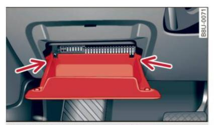
Fig. 169 Steering column area: Folding down cover
