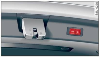
Fig. 28 Vehicles with convenience key: Closing and locking button in the rear lid
