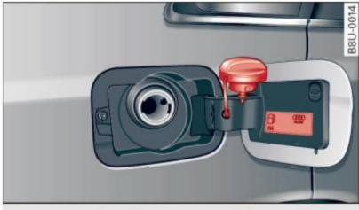
Fig. 141 Fuel filler flap with attached fuel cap
