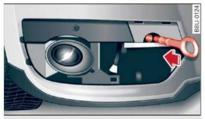
Fig. 174 Front bumper: Screwing in the towing loop
