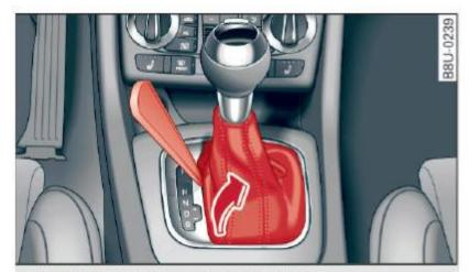
Fig. 90 Selector lever: removing the cover
