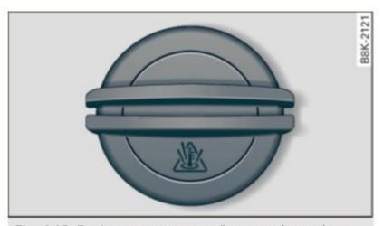
**Fig. 148** Engine compartment: Cover on the coolant expansion tank
