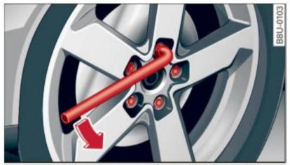
Fig. 164 Changing a wheel: loosening the wheel bolts
