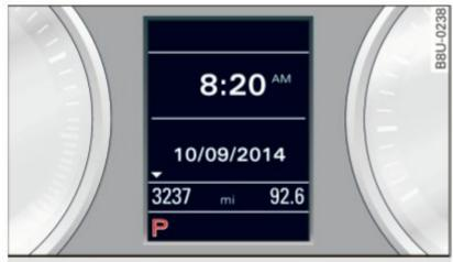
Fig. 86 Display in the instrument cluster: selector lever position
