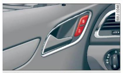
Fig. 22 Driver's door: power locking switch
