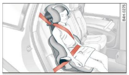
Fig. 129 Rear seat: child properly restrained in a booster seat
