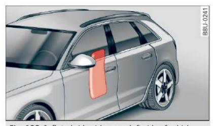
Fig. 122 Inflated side airbags on left side of vehicle
