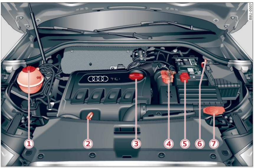
Fig. 145 Typical layout for containers and engine oil filler cap
