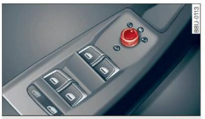
Fig. 41 Forward section of driver's armrest: power mirror controls
