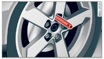
Fig. 168 Changing a wheel: alignment pin inside the top hole
