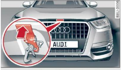
Fig. 144 Release lever under the engine hood
