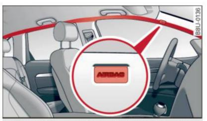
**Fig. 123** Side curtain system, driver's side: side curtain airbag location
