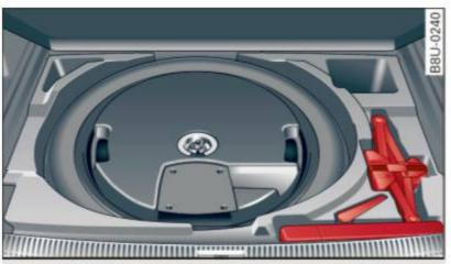
Fig. 158 Under the cargo floor cover: Tool kit, auxiliary tool and jack
