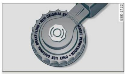
**Fig. 149** Engine compartment: Cover on the brake fluid reservoir
