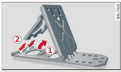
Fig. 159 Opening folding chocks
