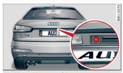
Fig. 98 Rear lid: Location of the rear view camera
