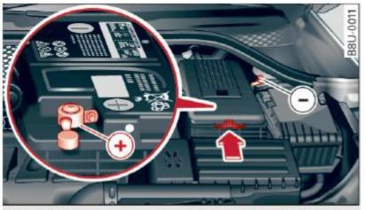
Fig. 171 Engine compartment: Connectors for jumper cables and charger
