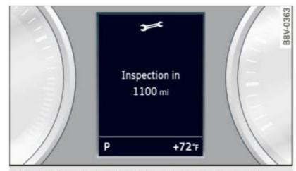
Fig. 15 Display: Service interval display (example)
