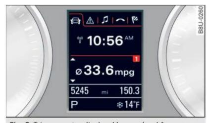
Fig. 8 Trip computer display: Memory level 1
