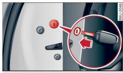
Fig. 24 Front passenger's door/rear doors: emergency lock
