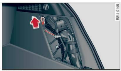
Fig. 142 Luggage compartment: Emergency opening of fuel filler flap
