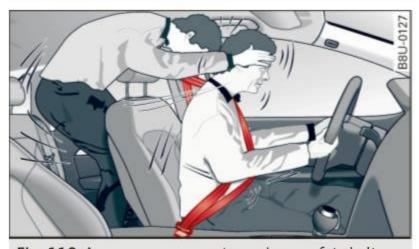
Fig. 110 A rear passenger not wearing a safety belt will fly forward and strike the driver
