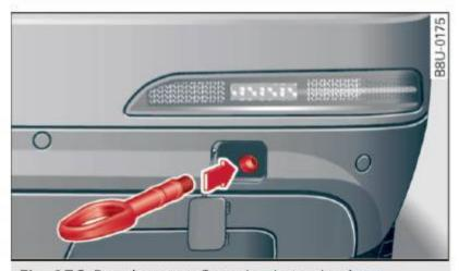
Fig. 176 Rear bumper: Screwing in towing loop
