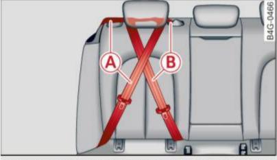
Fig. 125 Schematic overview: keep unused safety belts away from children in child safety seats. (A) - outer rear safety belt, (B) - center rear safety belt
