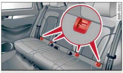
Fig. 132 Rear seats: lower anchorage bracket locations
