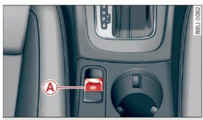
Fig. 77 Center console: parking brake
