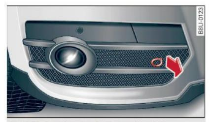
Fig. 173 Front bumper: Removing the cover
