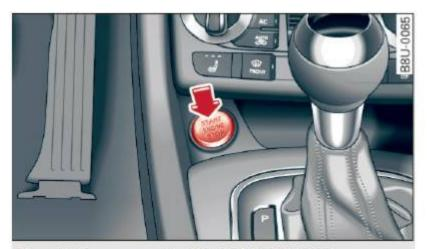
Fig. 75 Center console: START ENGINE STOP button
