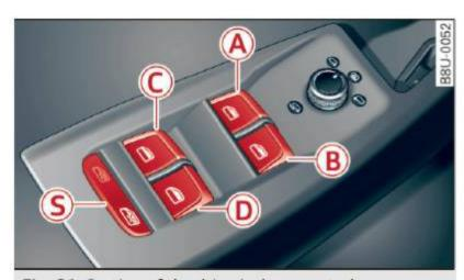
Fig. 31 Section of the driver's door: controls
