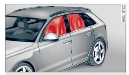
**Fig. 124** Illustration of principle: Inflated side curtain airbags on the left side
