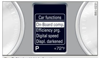
Fig. 7 Display: Vehicle functions menu
