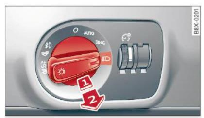
Fig. 34 Instrument panel: headlight control switch
