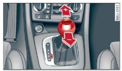
Fig. 88 Center console: shifting the gears manually
