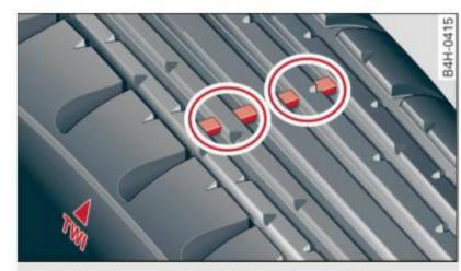
Fig. 154 Tire tread: tread wear indicators (TWI)
