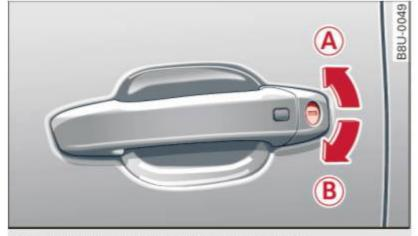
Fig. 32 Key turns for opening and closing
