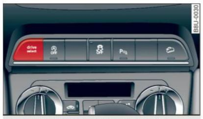
Fig. 84 Center console: Control for drive select
