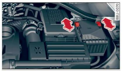
Fig. 170 Left side of the engine compartment: Releasing cover
