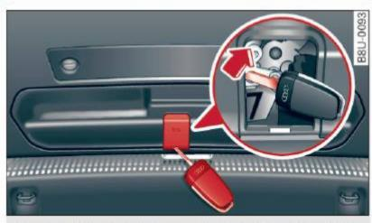
Fig. 29 Rear lid opening: access to the emergency release
