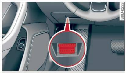
Fig. 16 Location of Data Link Connector (DLC)
